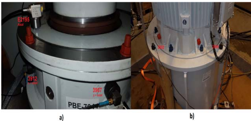
Figure 4. Vibration sensors mounted on locations according to API 610: a) Bearing housing, b) Driven mounting surface
