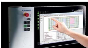
Converting edited drawings to macros on the production line
