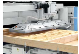
Fully automatic blow-in process for loose insulation material
