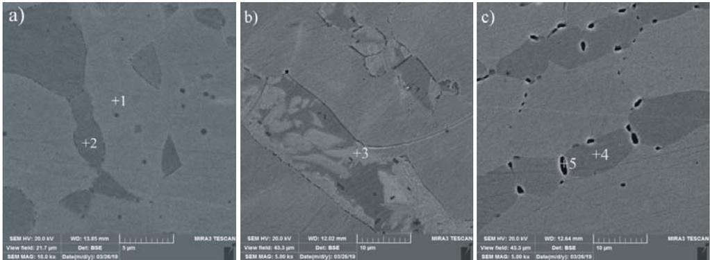
Figure 3. SEM-BSE image of annealed samples: a) 650, b) 750 and c) 1000 °C for 30 minutes, 10 000x
