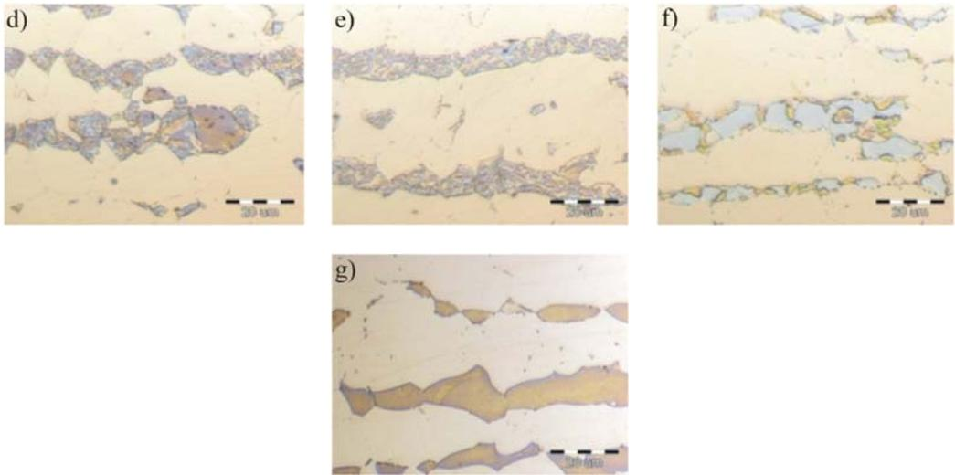
Figure 1. Microstructure of samples: a) solution annealed state and b-g) annealed at 550, 650, 750, 850, 950 and 1000 °C for 30 minutes, Murakami's reagent heated at 100 °C, 1000x
