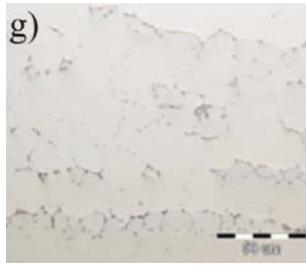
Figure 2. Microstructure of samples: a) solution annealed state and b-g) annealed at 550, 650, 750, 850, 950 and 1000 °C for 30 minutes, Murakami's reagent at room temperature, 500x
