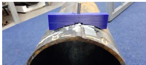
Figure 10. Prototype positioner mounted on the pipe DN200
