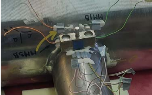
Figure 2. Tool positioner fixed at pipe surface [3]
