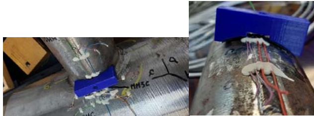
Figure 9. Prototype positioner mounted on the pipes
