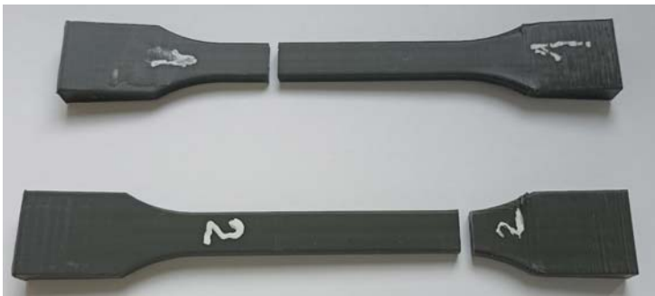
Figure 10. Fractured specimens after tensile testing.
