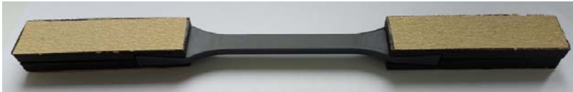
Figure 7. The specimen positioned into the grips with glued sanding papers.
