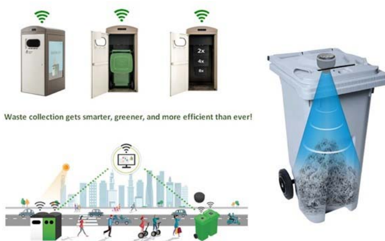
Figure 2. Smart bins rely on sensors to minimize the transportation costs [11]
