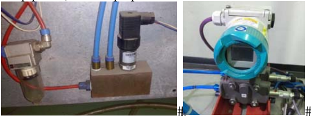
Figure 4. D8A-02A pressure transducer and pressure gauge.
