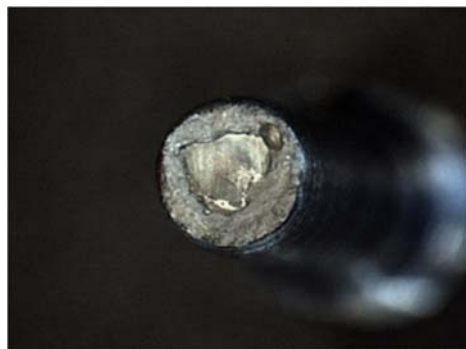
Figure 8. Example of the fracture surfaces of the tensile test pieces for Sample No.2, 6,3x
