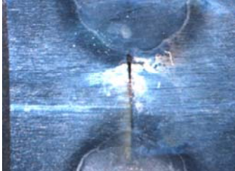
Figure 4. Example of a welding defect in the form of an incomplete penetration, 8x
