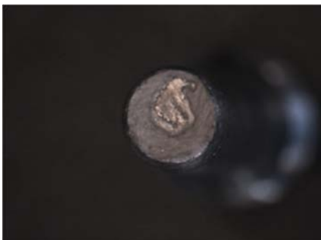
Figure 7. Example of the fracture surfaces of the tensile test pieces for Sample No.1, 6,3x
