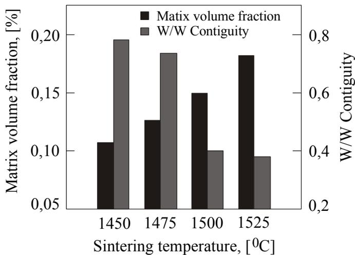
FIGURE 3. THE VARIATION OF THE FRACTION INTO THE MATRIX VOLUM, AND OF THE CONTIGUITY W/W, OF THE HEAVY ALLOY BASED W SINTERED IN 2 STEPS DEPENDING ON THE SINTERING TEMPERATURE, FROM 1450 °C AT 1525°C.
