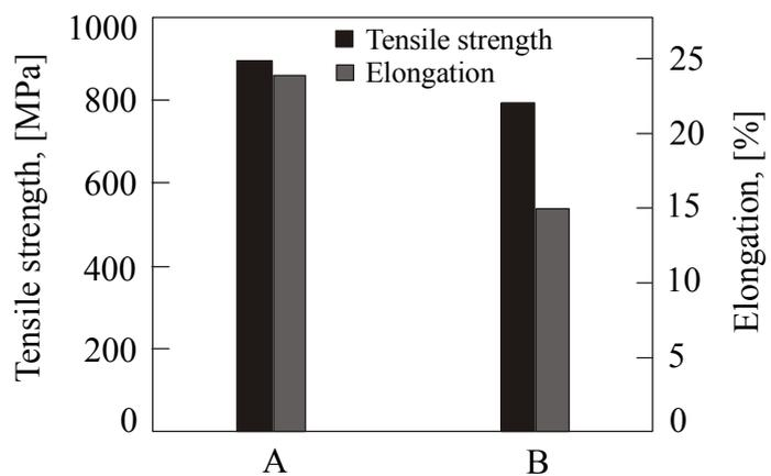
FIGURE 4. THE VARIATION OF THE TENSILE AND THE TENSILE STRENGTH FOR: A) – THE AGW CONVENTIONAL SINTERED WITH LIQUID PHASE, B) - AGW SINTERED IN 2 STEPS, INCLUDING A SINTERING WITH LIQUID PHASE AT 1500 °C FOR 60 MIN.
