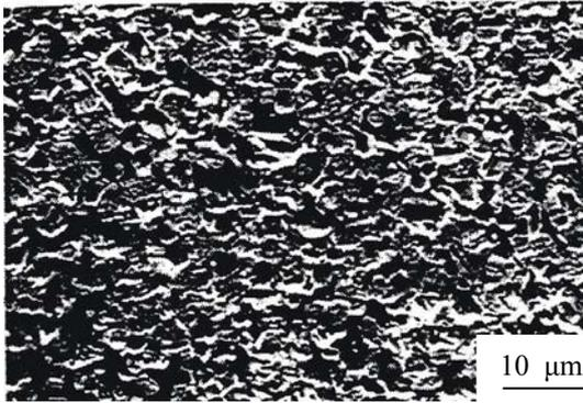
FIGURE 1. THE SEM IMAGE OF THE MICROSTRUCTURE OF THE HEAVY ALLOY BASED W, 90W-7NI-3FE SINTERED AT 1275 °C.
