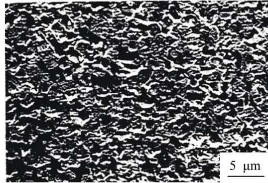
FIGURE 2. THE SEM IMAGE OF THE MICROSTRUCTURE OF THE HEAVY ALLOY BASED W 90W-7NI-3FE SINTERED IN SOLID STATE AT 1275 °C.
