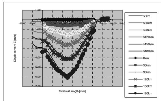
Figure 6. The axial displacement of the sidewall for 27° breaker angle (s-simulation, m- measurement)
