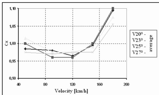
Figure 7. The experimental  $C_x$  versus velocity for different breaker angles
