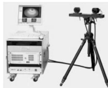
Figure 2. Optical system Aramis
