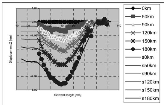
Figure 4. The axial displacement of the sidewall for 23° breaker angle ( s-simulation, m- measurement)
