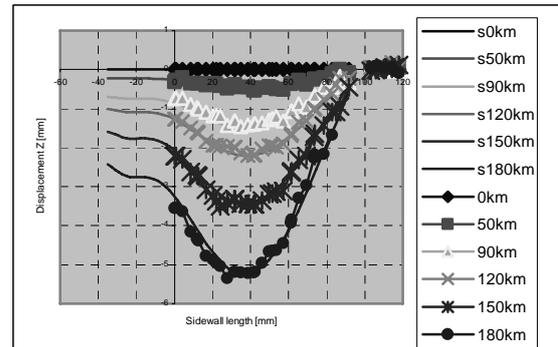
Figure 5. The axial displacement of the sidewall for 25° breaker angle (s-simulation, m- measurement)
