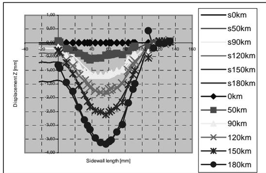
Figure 3. The axial displacement of the sidewall for 20° breaker angle (s-simulation, m- measurement)
