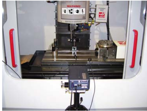
Figure 1. Measurement using Laser interferometer
