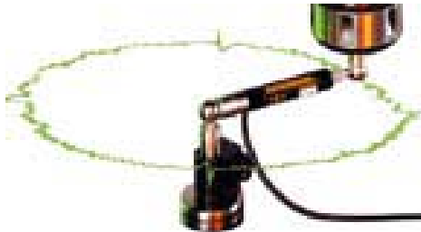
Figure 3. Principle of measurement with Renishaw equipment QC10 Ballbar
