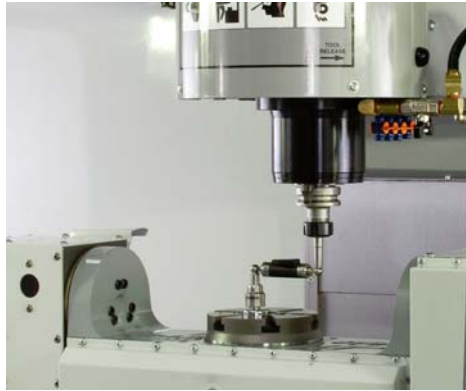
Figure 2. Measurement of geometrical inaccuracy of CNC machine tool with QC10 Ballbar
