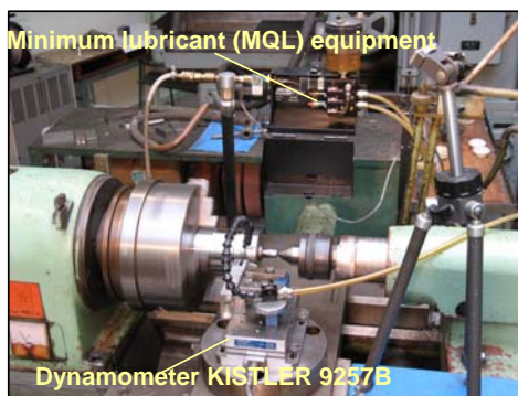
Figure 4. Experimental measuring layout for diamond burnishing
