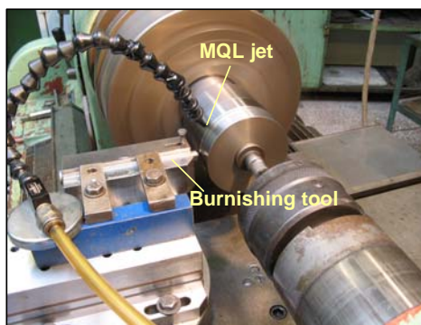
Figure 4. Experimental measuring layout for diamond burnishing
