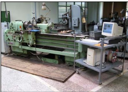
Figure 1. The measuring system and work area used for force measurements
