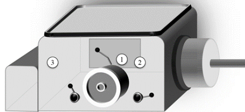
Figure 1. Position of thermocouples on the front side of main gearbox housing
